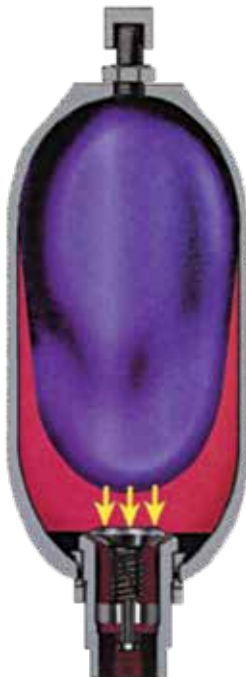
The poppet closes, trapping oil in the accumulator
