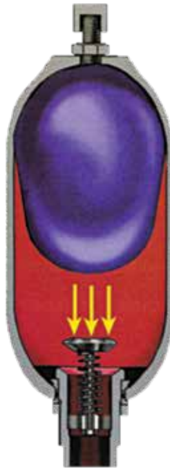
Oil discharging from the accumulator causes a pressure drop at the poppet
